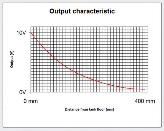
The Picture above depicts the analogue output volts related with the distance between the strip and the tank floor, considering 0 mm the tank floor (generally granite or marble domes).
